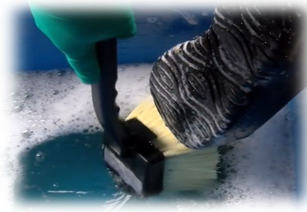
Figure 2: Pay special attention to scrubbing the threads with soap and water to remove all debris.
